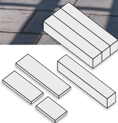
Barn Plank has the look of weathered white pine, with soft edges, deep splits and detailed grain on all sides. Made from 10,000 psi wet cast concrete, Barn Plank will never warp, splinter or rot.
